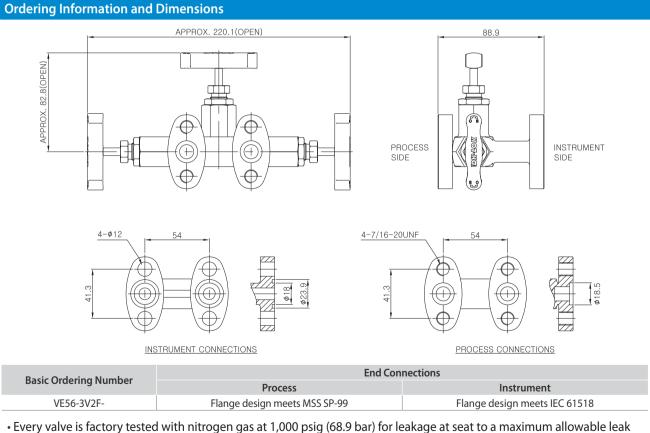
• Every value is factory tested with nitrogen gas at 1,000 psig (68.9 bar) for leakage at seat to a maximum allowable lea rate of 0.1 SCCM. The packing is tested with nitrogen gas for no detectable leakage.
