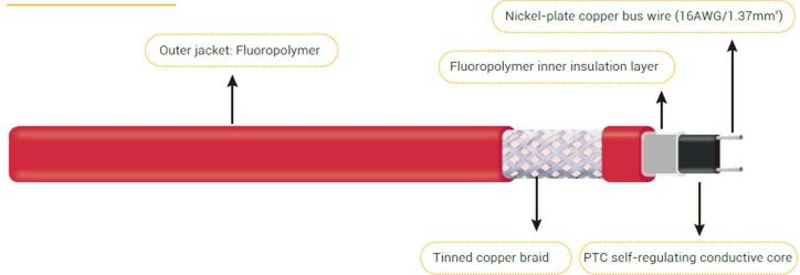
The extruded core tape, which made by parallel nickel-plate copper bus wire and PTC semiconductor polymer heating material, and inner insulation layer of fluoropolymer are added to tinned copper braid and the outer jacket form a complete structure of TSCR heating cable, in which the outer jacket can be made of fluoropolymer material (CT).
