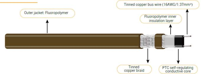
The extruded core tape, which made by parallel tinner copper bus wire and PTC semiconductor polymer heating material, and inner insulation layer of fluoropolymer are added to tinned copper braid and the outer jacket form a complete structure of TPCR heating cable, in which the outer jacket can be made of fluoropolymer material (CT).
