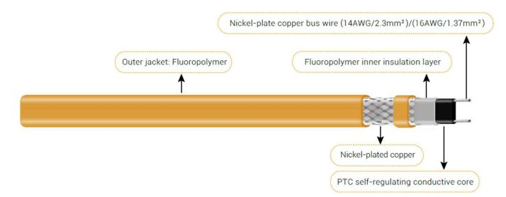
The extruded core tape, which made by parallel nickel-plate copper bus wire and PTC semiconductor polymer heating material, and inner insulation layer of fluoropolymer are added to the nickel-plated copper and the outer jacket form a complete structure of TUCR heating cable, in which the outer jacket can be made of fluoropolymer material (CT).
