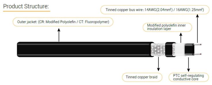
The extruded core tape, which made by parallel tinner copper bus wire and PTC semiconductor polymer heating material, and inner insulation layer of modified polyolefin is added to tinned copper braid and the outer jacket form a complete structure of TRCR heating cable, in which the outer jacket can be made of modified polyolefin material (CR) or fluoropolymer material (CT) according to different application or area.
