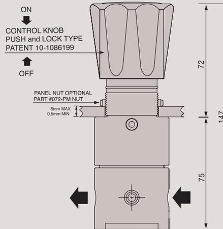
outside or minute vibration at the gas pipeline. You can prevent the self-changing of pre-set value just by pushing the handle and reset the value freely by drawing the handle. DRASTAR has created and applied patent for this push and lock system for DRASTAR regulators (patent number 10-1086199).
